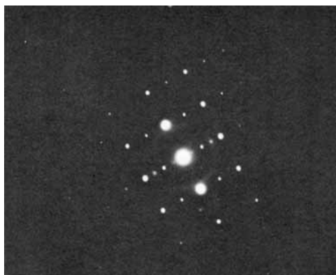
Fig. 9. Electron diffraction pattern of black area at arrow tip in Figure 8.
